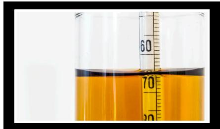
To ensure the solution contains the appropriate amount of active ingredient (Ethanol), use a Hydrometer. The reading should be 0.879 (+/- .02 at 20 degrees).
